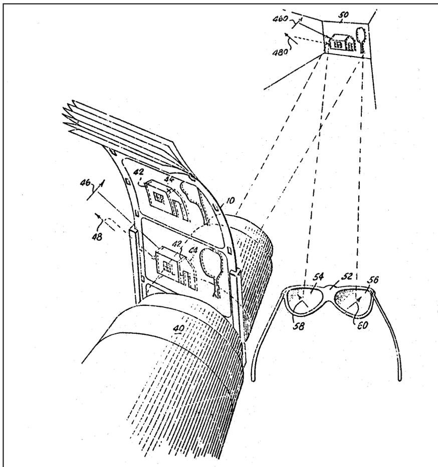
Figure 2. Vectograph projection. A single film contains both left and right images with each having the ability to polarize light. This drawing is from a 1942 patent by Land.
