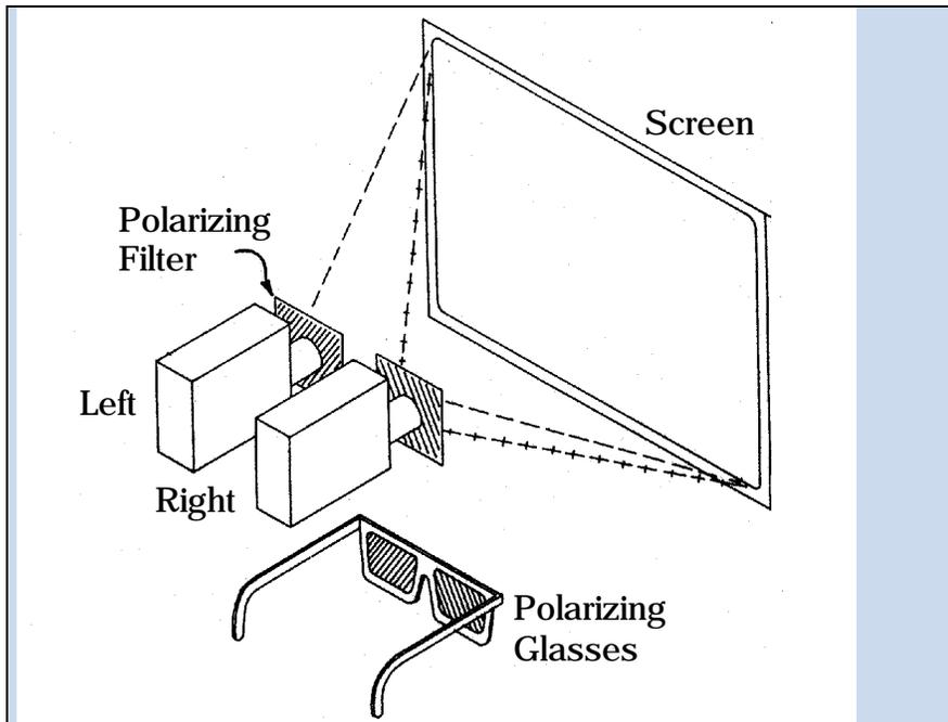
Figure 1. Polarization image selection. Sheet polarizers are used over the projection lenses and as analyzers in eyewear. Projection screen must conserve polarization.
