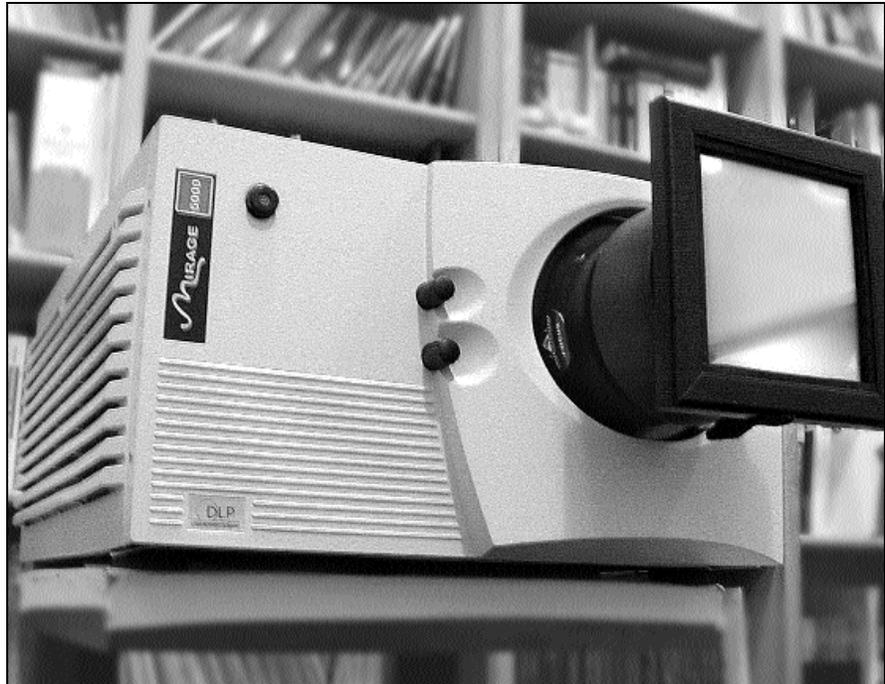
Figure 4. ZScreen mounted on a Mirage projector.
