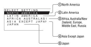
2 Press the + or – button to select the area where you intend to use the unit and press the ENTER button.
