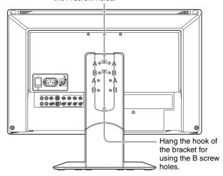
**5** Secure the arm with four screws.
